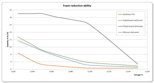
Foam reduction capability of different defoaming agents in a reference mortar of Pentachem.
