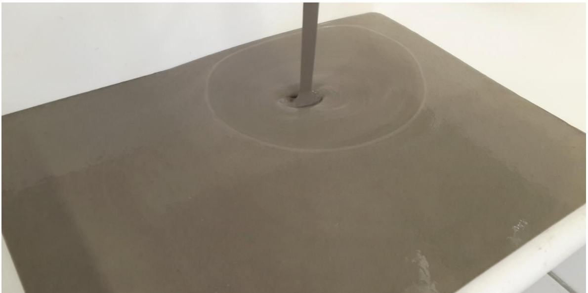
Picture of a self-levelling screed made with Pentaflow SA.2
