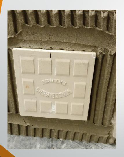
Vertical slip resistance test for the definition of T class:
